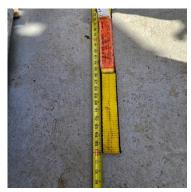
An offshore crew was looking into why their lifts were not level when performing crane operations. The finding was that a nylon strap they were using was eight feet long and labeled ten feet long. The strap was destroyed at the customer's request and a Non-Conformance Report was performed and sent in.
