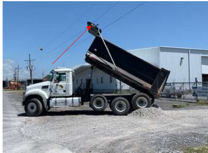
Power Line Making Contact with Truck
