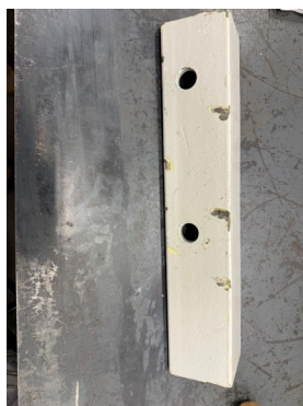
3" x 3" x 1/4" angle-iron support - 16" long, 9.6 lb.
