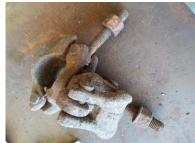
We recommend oiling the clamps (especially when in an offshore environment) to assist with longevity. Also, here is a brief checklist you can use to improve the longevity of your scaffolding parts.
