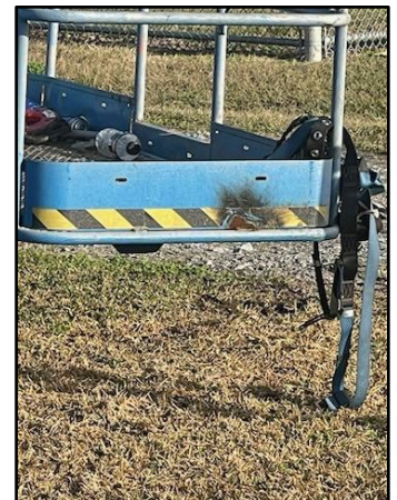
GIS Man-Lift Power Line Contact
