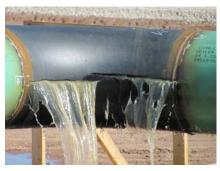
Hydrostatic testing is an important process to check the strength of piping. However, failure or disregard of the strict safety rules can lead to severe injury or death. Please remember these tips when conducting hydrostatic testing.
