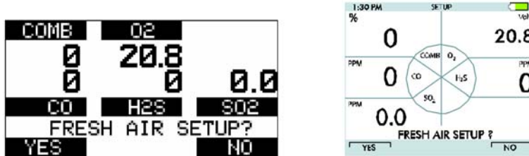
Figure 3-1. Fresh Air Setup
