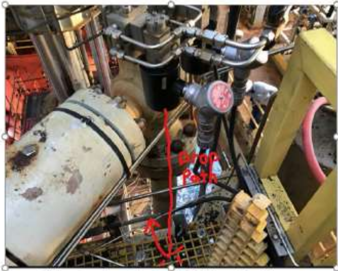
1.6 kg piece of metal sclenoid (DO) drops 5 feet from wellhead to dry crows nest on A1 dry tree and bounces down off the grating
