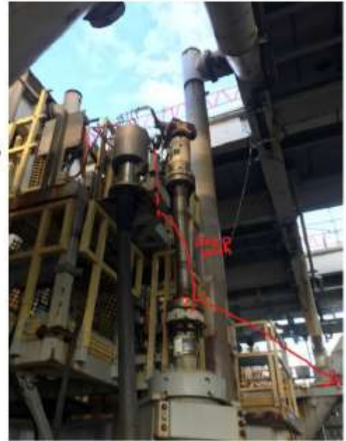
DO then falls another 10 feet and bounces off a flange in the well bay area
